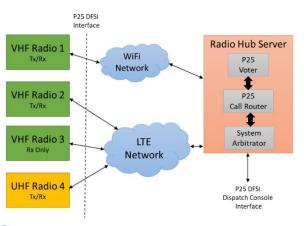
Calls are routed based on P25 TGID or NAC codes. This allows partitioning of calls based on group communication needs. The ability to assign priorities based on TGID, NAC and or a communication port ensure higher priority calls are transmitted.
